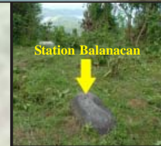
Station Balanacan mark is intact on a hill locally known as Mataas na Bundok (upper left) with reference marks nearby (right pictures)
